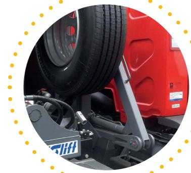
**Hydraulic foldable spare wheel carrier located behind the cabin**
