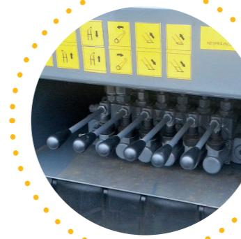
**Hydraulic valve block. STOP button and fast off-load incl.**
