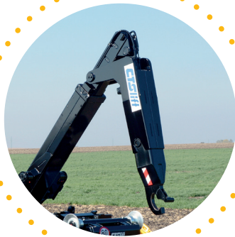
Combined sliding and articulated hook arm Potence coulissante et articulée
