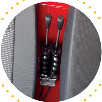
Bowden cable in-cab control Bowdencommande
